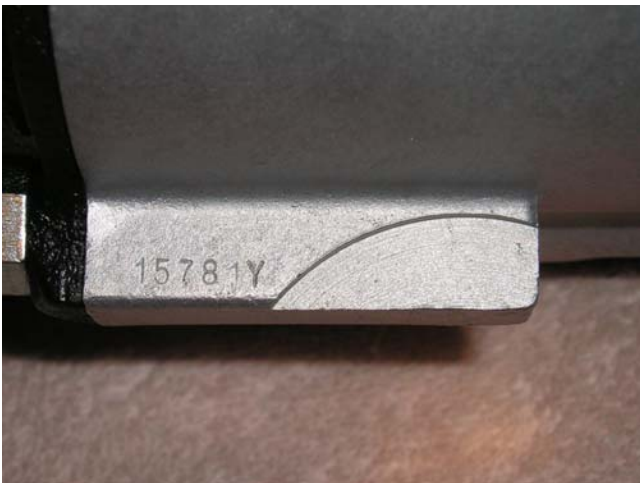
Note the pump stamping date, 15781Y, decodes as the 157th day of 1968, with a Saginaw plant code of 1Y. In the case of 1968 pumps, original pumps have been found with this julian stamping on the machined flange shown here or right next to the machined flange as shown here in our photo.
