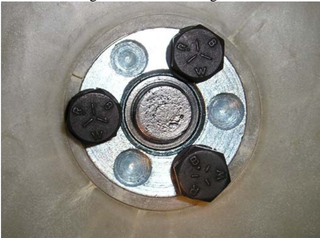
Close up showing the original restored "RBW" pulley mounting bolts.
