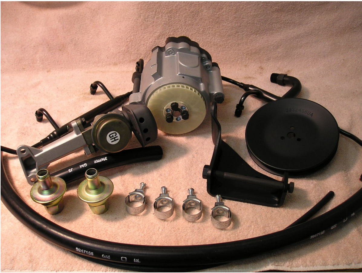
Here is one of our restored NOS smog systems for a 1970 396 or 454. It's complete and ready to install.
