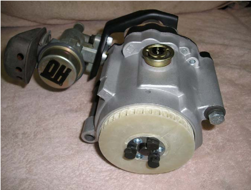
Restored original white fan pump w/ NOS DH diverter valve.
